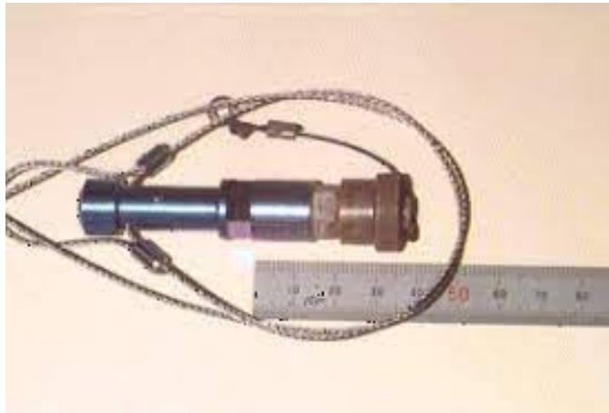
Figure III.23. Pyrotechnic actuator for car airbags
