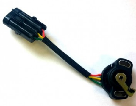
Figure II.36. The throttle position sensor (potentiometer)
